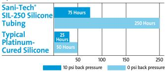
The performance of tubing in peristaltic pumping applications is affected by the conditions of use and equipment utilized, along with size and wall thickness of the tubing tested. The data above is presented for information only and should not be utilized for specification purposes.
